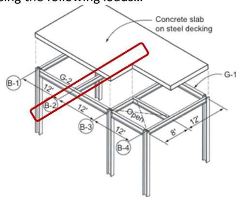
) Isometric view of partial steel framing arrangement
