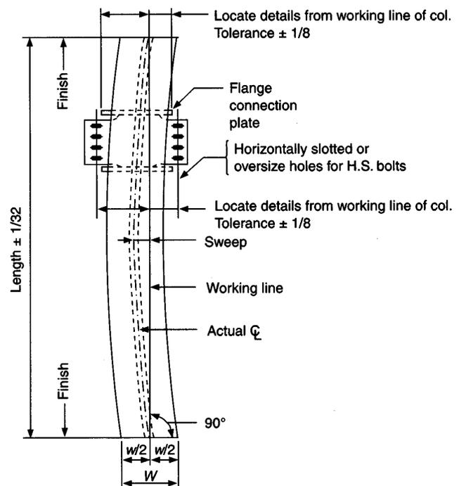
Figure 5. Adjustments for column sweep in beam-to-column connections.
