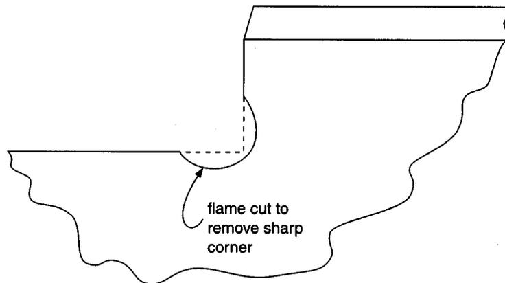
**Figure 1.** Correction of square-cut copes.
