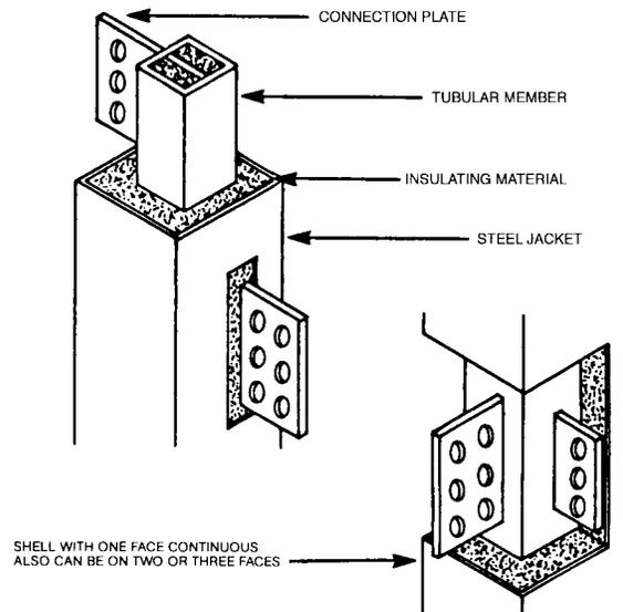
Figure 40. Typical connections in a continuous shell
