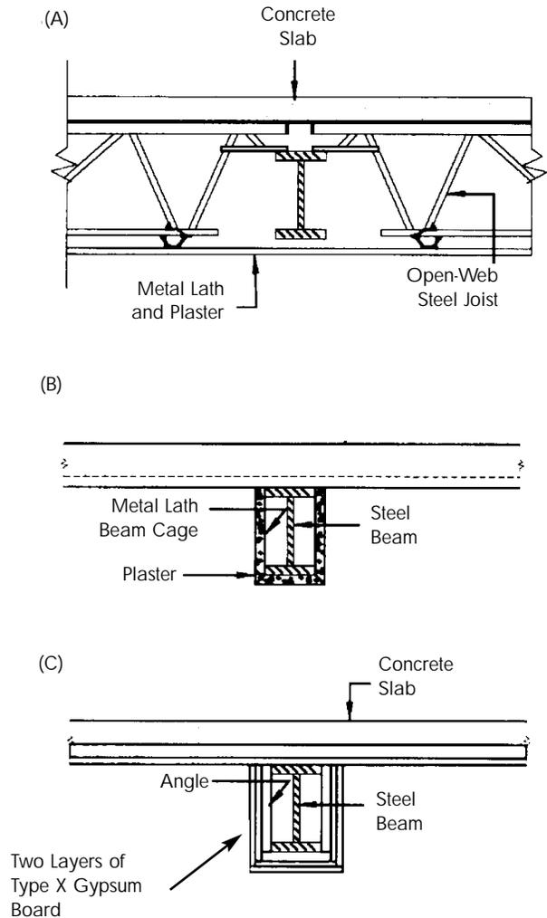
**Figure 31.** Some methods for applying gypsum as fire protection for structural steel: (a) open-web joist with plaster ceiling; (b) beam enclosed in a plaster cage; (c) beam boxed with wallboard. Illustration courtesy of the Gypsum Association, *Fire Resistance Design Manual*.
