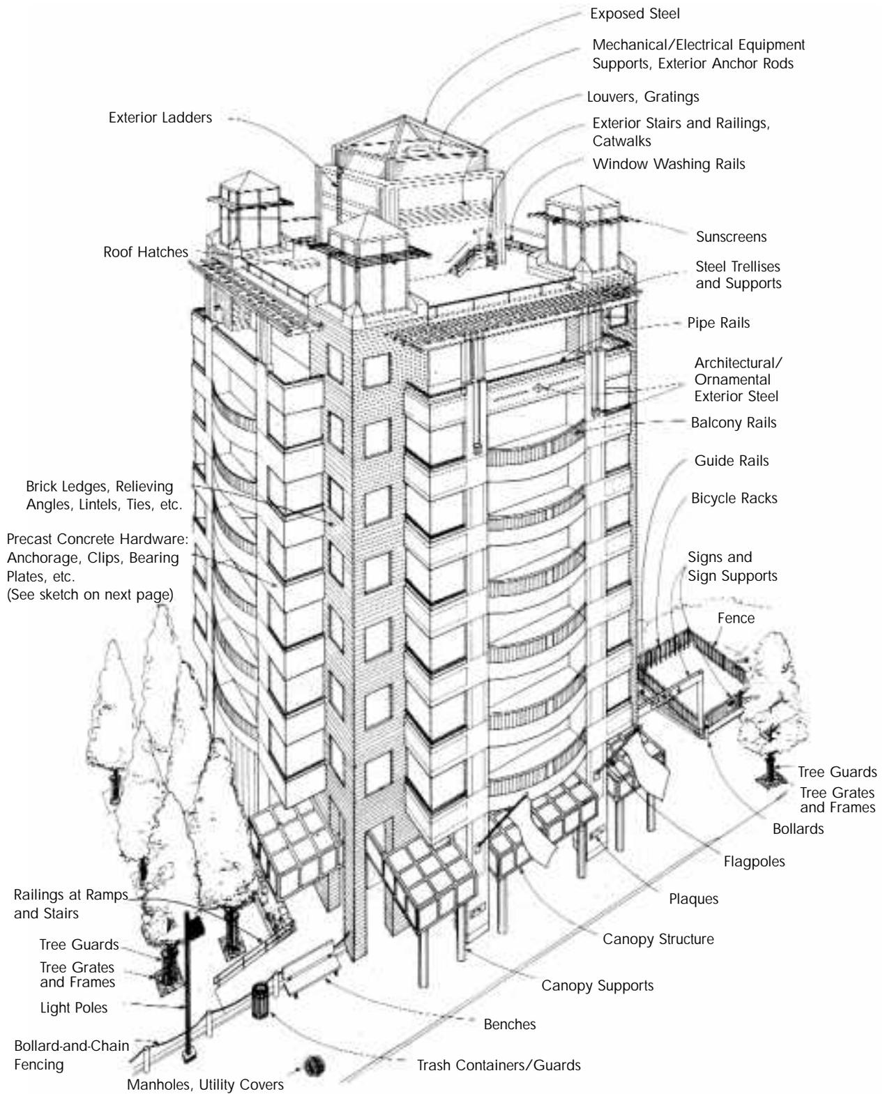
Figure 24. High potential corrosion areas of high-rise buildings
