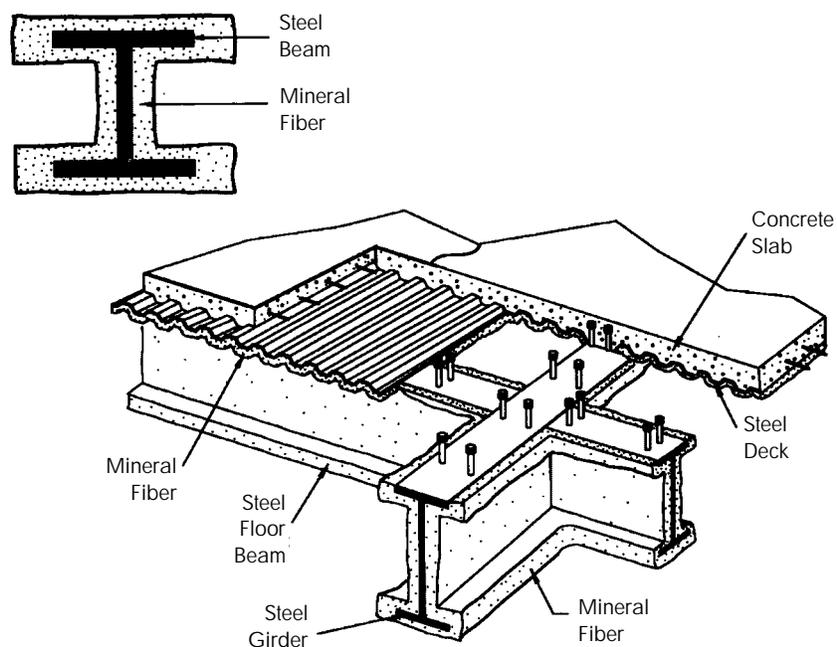
**Figure 32.** Mineral fiber spray applied to beam and girder floor system with steel floor deck supporting a concrete slab. Illustration courtesy of the American Iron and Steel Institute, *Designing Fire Protection for Steel Beams*.
