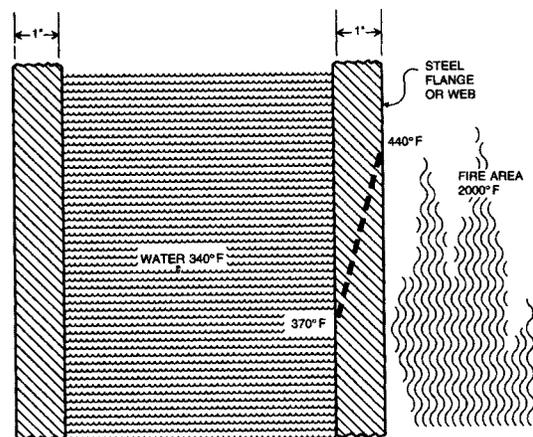
**Figure 35.** Tubular steel columns filled with water for fire resistance with temperature variation during exposure to fire. Illustration courtesy of the American Iron and Steel Institute, *Fire Protection Through Modern Building Codes*.
