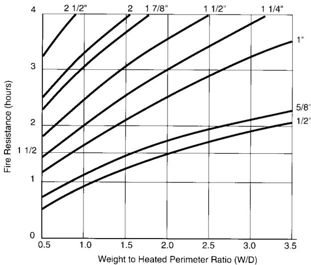
**Figure 30.** Variation in fire resistance of structural steel columns with weight to heated perimeter ratios and various gypsum wallboards. Illustration courtesy of the American Iron and Steel Institute, *Designing Fire Protection for Steel Columns*.
