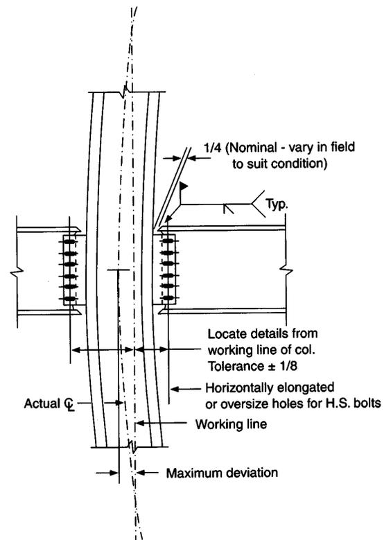
Figure 4. Adjustments for column curvature in beam-to-column connections.
