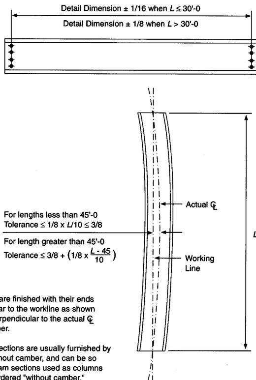
Figure 2. Beam and column fabrication tolerances
