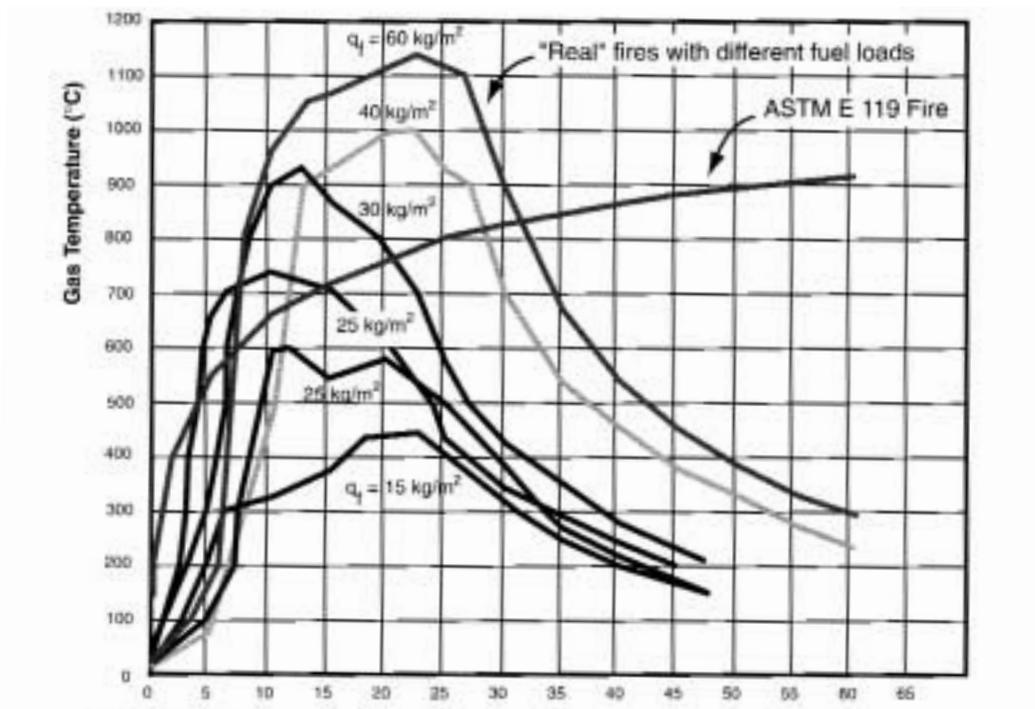
Figure 28. Time/temperature curves for various fire exposures
